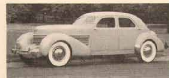
Cord: an American design contrasting a coffin-shaped hood with separate streamlined fenders.
