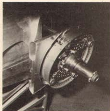
As displayed in the Donington Museum, this Cisitalia has been assembled as far as possible from parts. Rear brake with drum removed is shown above.
