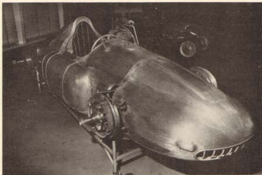
As displayed in the Donington Museum, this Cisitalia has been assembled as far as possible from parts. Rear brake with drum removed is shown above.
