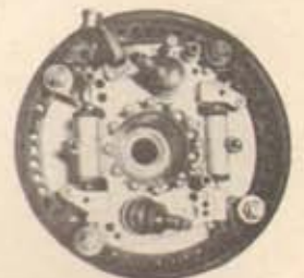
Originally published pictures of the completed chassis, a fairly fully ancilliaried engine and a front brake assembly seen with the backplate removed.
